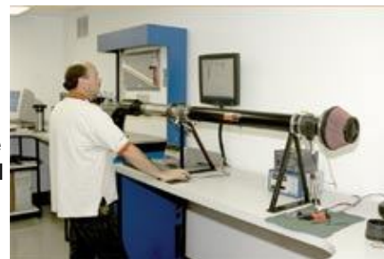
MAF Sensor Test Bench
