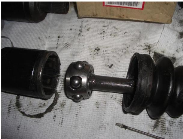
Step 16: Removal of CV bearing assembly from the axle shaft. The bearing assembly consists of three parts, bearing cage, bearing race and steel balls. You will also notice there is no part number reference to these three parts which are part of the inboard joint assembly and is Honda part# 42220-HE0-003 for the 1989 FI400 and superseded to 42220-HE0-013 for the 1990 FI400. This part is still available as of 12-12-2013.
