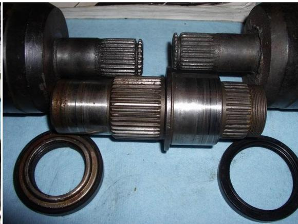
Before moving onto the boot replacement let's take a look at the knuckle assemble. Now that we have it off the pilot and benched and the axle has been removed we need to take a closer look at the hub/axle seal lip where the axle sets inside of to see if it's dry or tore.
