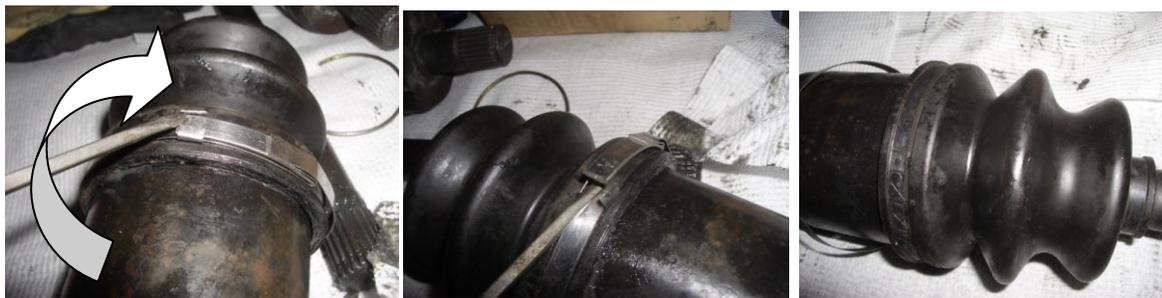
Step 15: This will allow you to slide the CV boot (#14) towards the outboard joint. This will allow you to remove the internal keeper (stop ring) inside the inboard joint (#4) and allow the CV cup to slide off the axle assembly.
